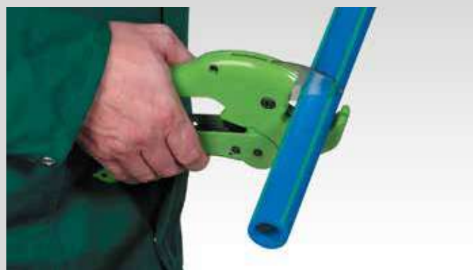
Cutting of the pipe
